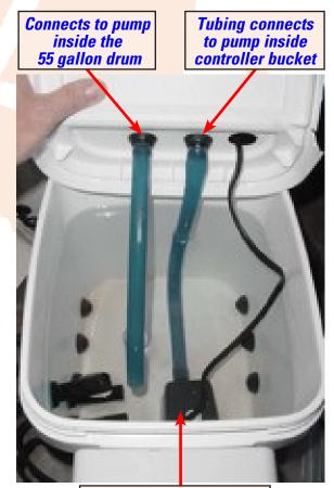
Stick pump to the side of the controller with the opening facing down.
